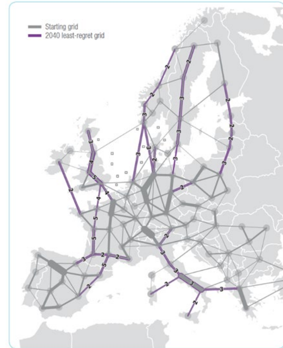
The most robust Europe wide grid architecture for a low carbon future 2040 from e-Highways
