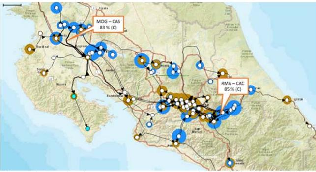
Figure 6: Results for wet year, wet season, high wind / peak load: No overloaded lines, highest loadings occur on the lines Mogote – Canas and Rio Macho – Cachi during double contingencies in the respective areas.
