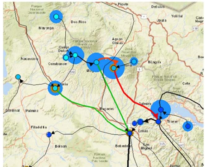
Figure 4: Overloading of >150 % on lines Mogote - Miravalles and Miravalles - Arenal (shown in red) in case of a double contingency and 470 MW of additional wind installed at the five best wind locations.
