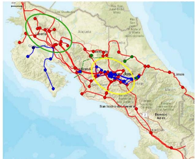
Figure 2: Costa Rican Transmission Grid, 230 kV in red, 138 kV in blue. The area in Guanacaste circled in green provides most of the generation during the dry season, while most of the load is located within the yellow circle.
