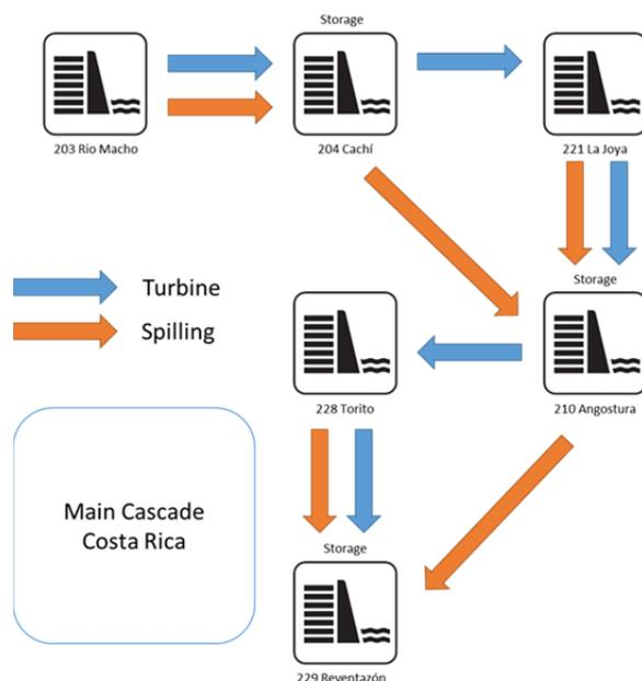
Figure 1: 883 MW cascaded hydro scheme on the Macho and Reventazón rivers.
