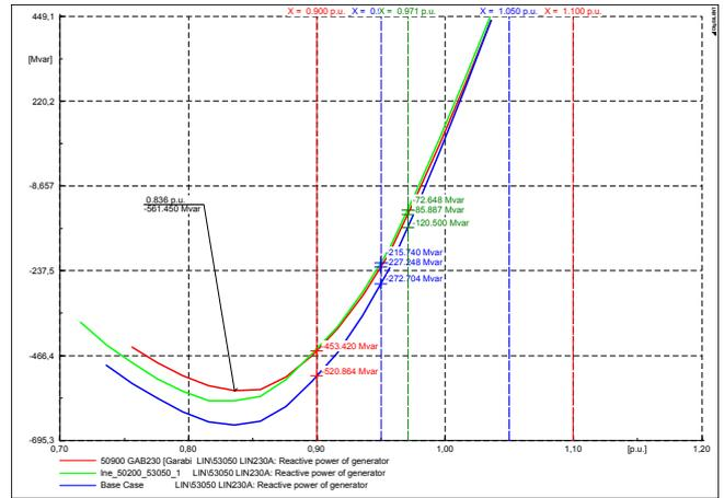
Figure 7: Q-V curve at bus bar Lindora 230kV for the base case (n-0) and the critical contingencies Garabito 230kV (bus bar fault) and 230kV line Lindora-Arenal under peak (day) demand in the dry season
