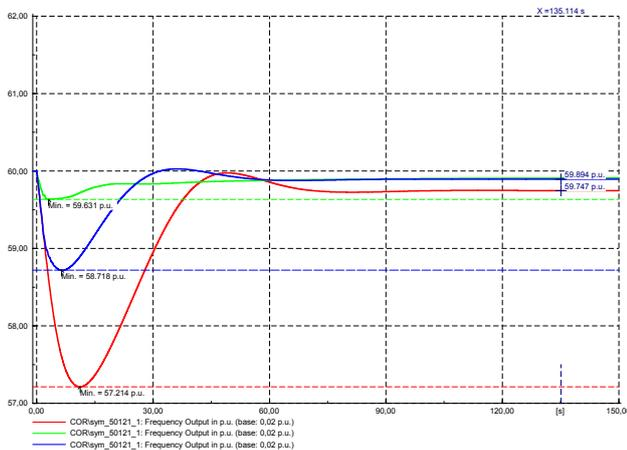
Figure 9: Primary frequency response for the loss of 110MW of generation in Pirris. In Green: Costan Rican system interconnected to the SIEPAC; in Blue: isolated operation with a total load shedding of 66MW, in Red: isolated operation (without load shedding scheme.)
