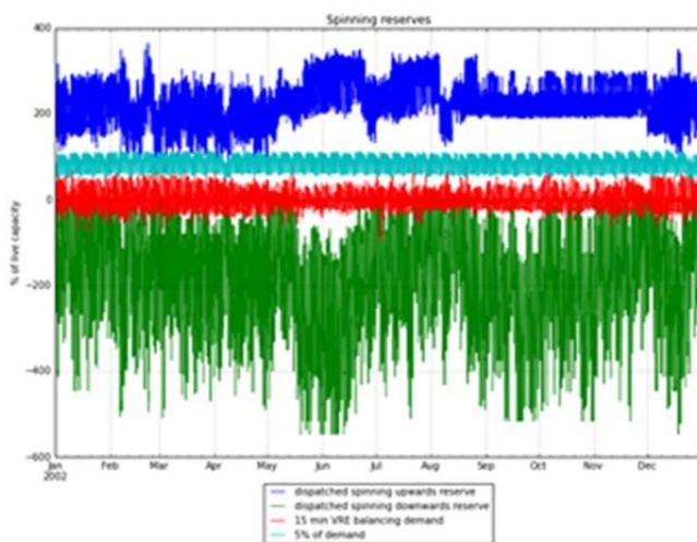
Figure 3: Dispatched reserve power and VRE fluctuations across one year, simulation result.
