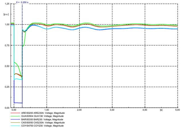
Figure 8: Dynamic voltage recovery after a bus bar fault at Garabito 230kV for peak (day) demand in the dry season.
