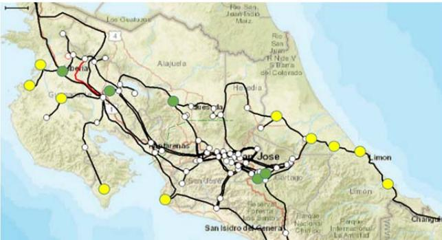
Figure 5: Installations of new centralized PV (yellow) and wind power plants (green) for the 2024 VRE Advanced scenario.
