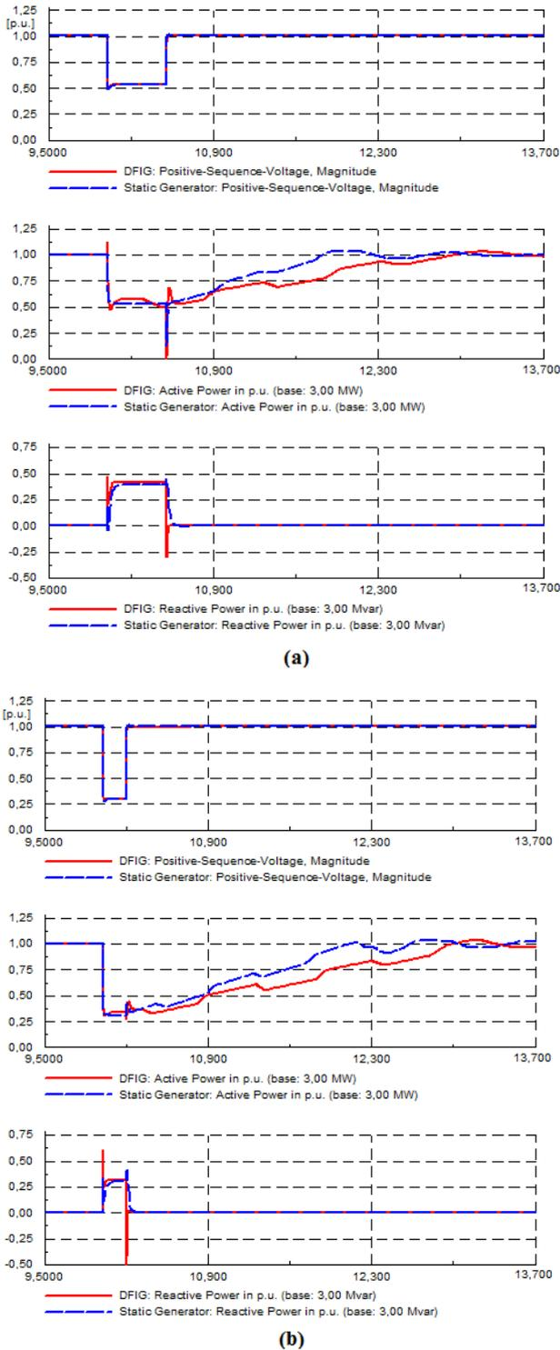
Fig. 4. FRT simulations with Type 3 generic model (blue dashed line) and manufacturer model (red solid line), (a): 50 % residual voltage, (b): 25 % residual voltage
