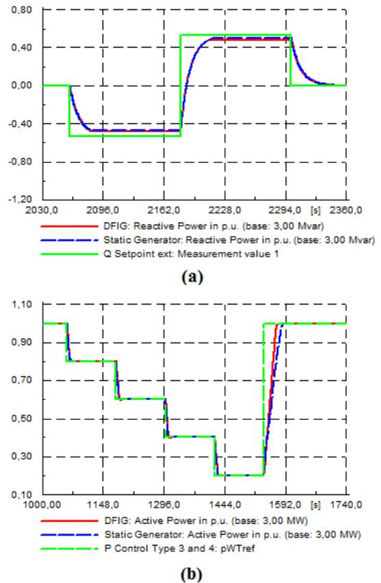
Fig. 5. Reference values steps with Type 3 generic model (blue dashed line) and manufacturer model (red solid line), (a): Reactive power (b): Active power, the simulations were conducted separately
