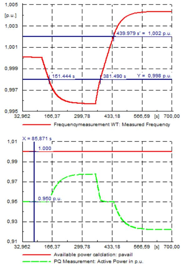
Fig. 3. Reaction of the WT to frequency deviations with activated Delta Control
