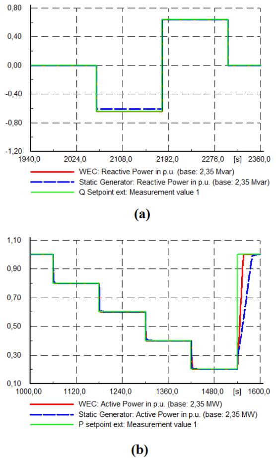
Fig. 7. Reference values steps with Type 4 generic model (blue dashed line) and manufacturer model (red solid line), (a): Reactive power (b): Active power, the simulations were conducted separately
