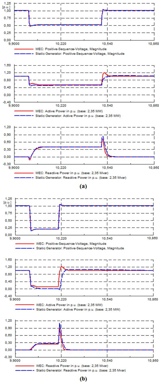
Fig. 6. FRT simulations with Type 4 generic model (blue dashed line) and manufacturer model (red solid line), (a): 50 % residual voltage, (b): 25 % residual voltage
