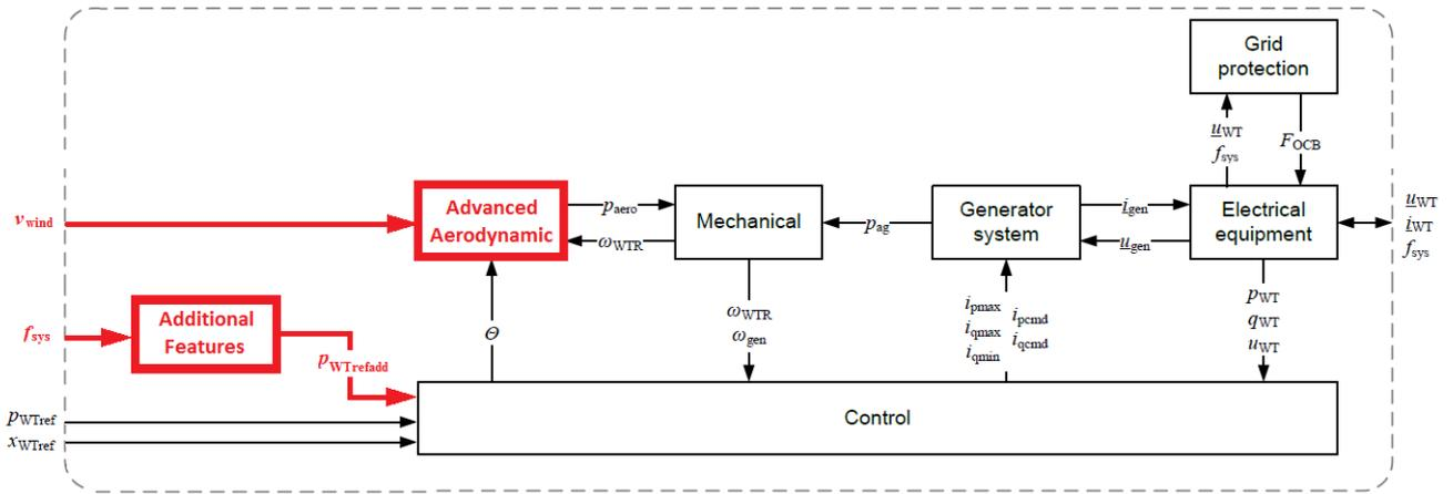
Fig. 1. Modified IEC control structure of type 3 WT, new or modified blocks or signals are marked in red and bold
