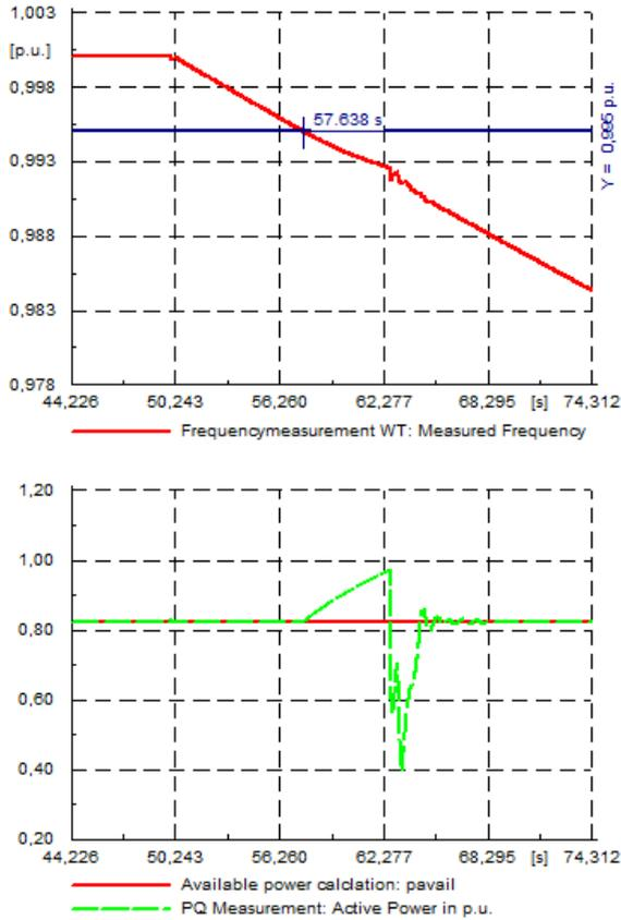
Fig. 2. Reaction of the WT to Underfrequency with activated Emulated Inertia
